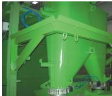
Cement and Water Weighing system
